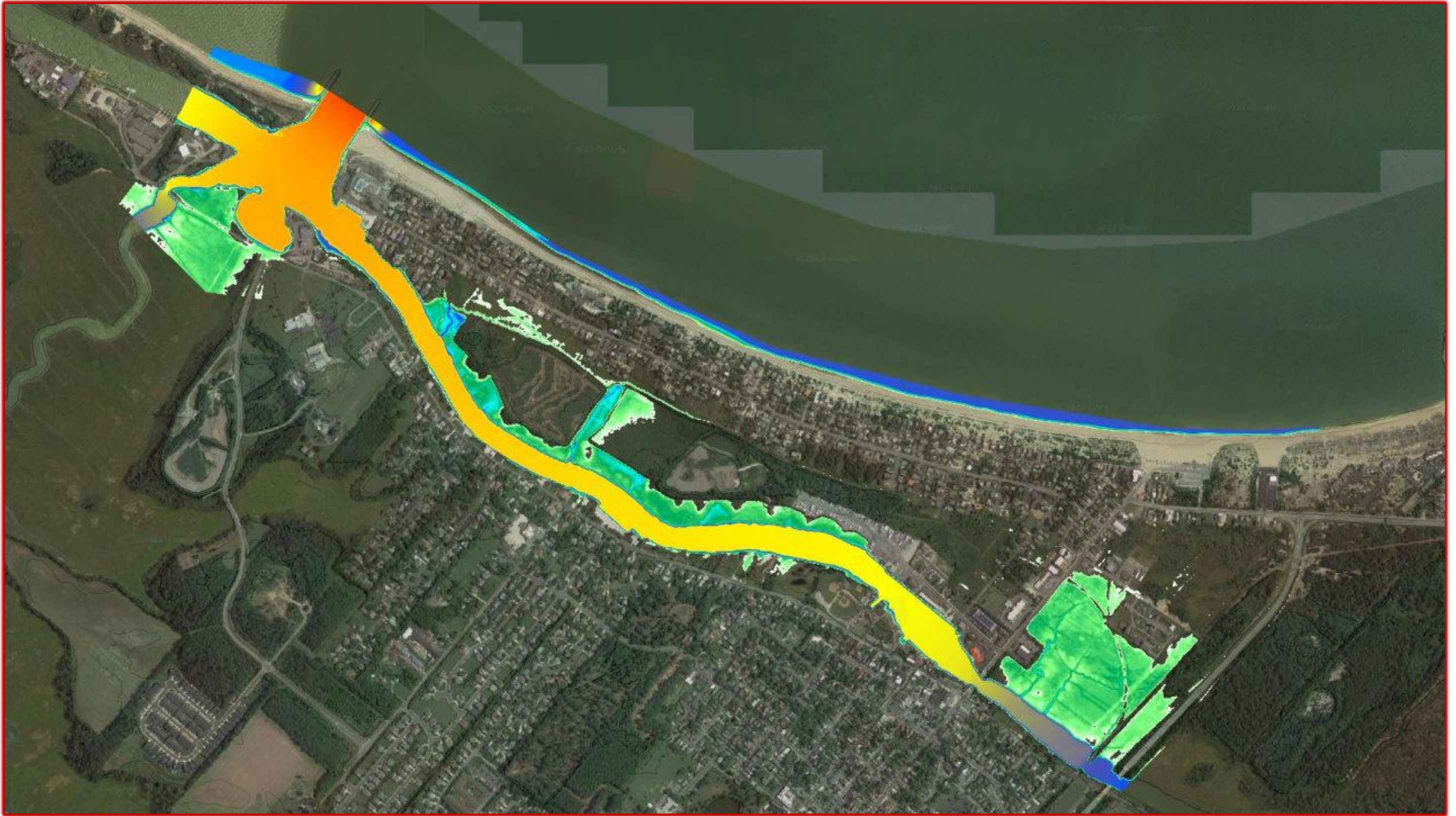
Maximum Tide Elevation 5.0 – Post-Berm Installation Model
