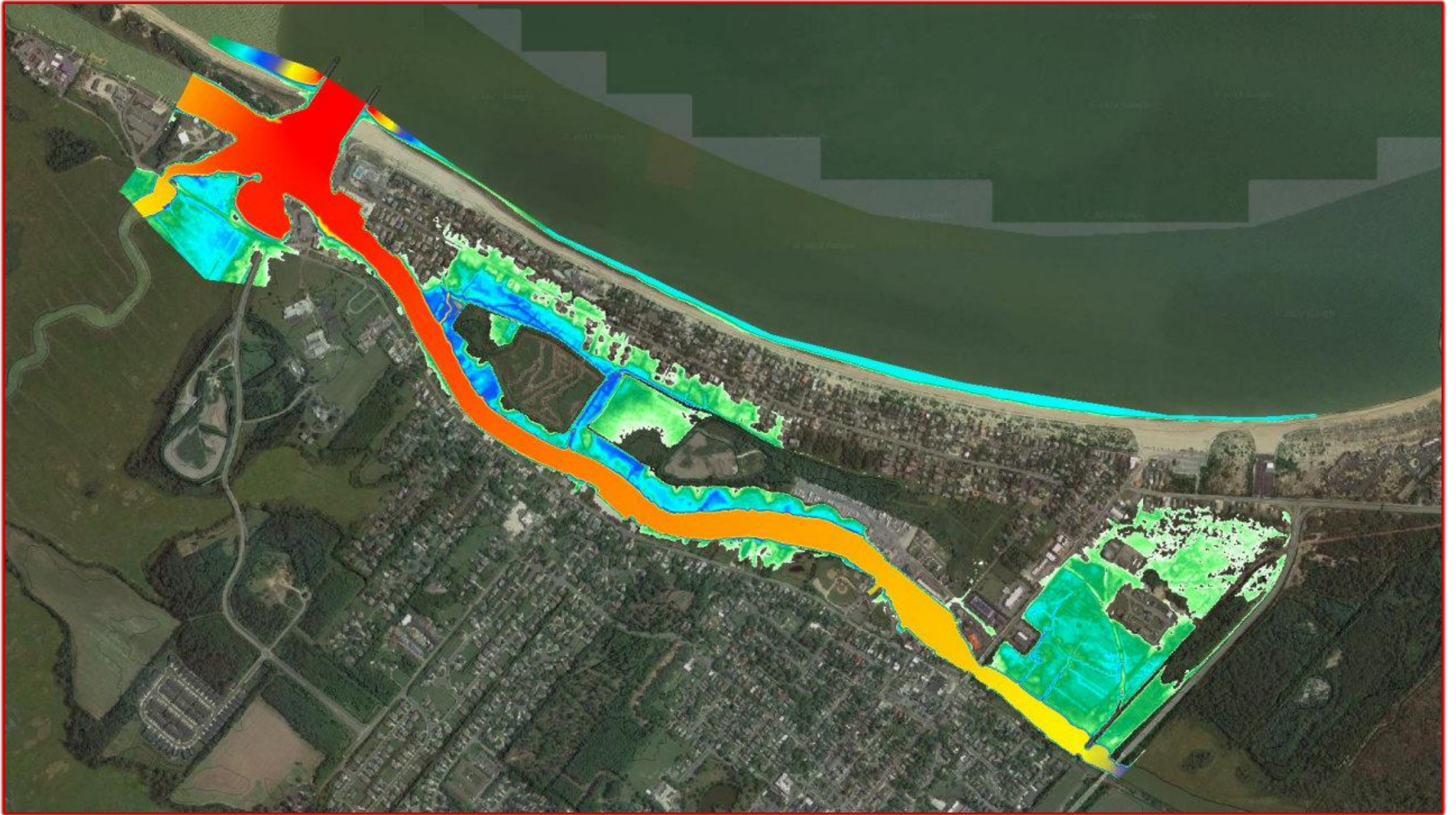
Nor'easter January 1998 – Post-Berm Installation Model
