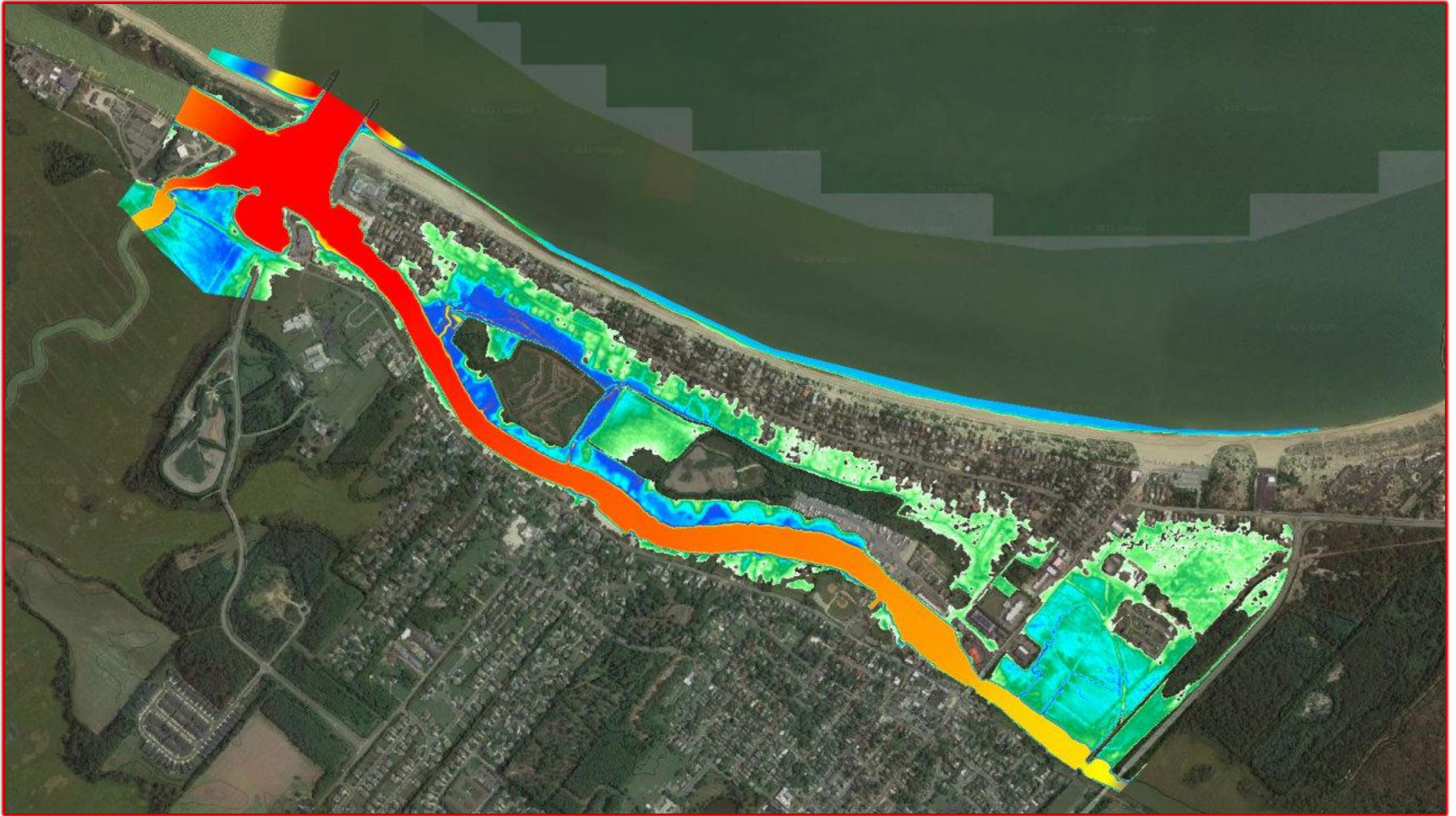
Winter Storm Jonas Flood – Post Berm Installation Model
