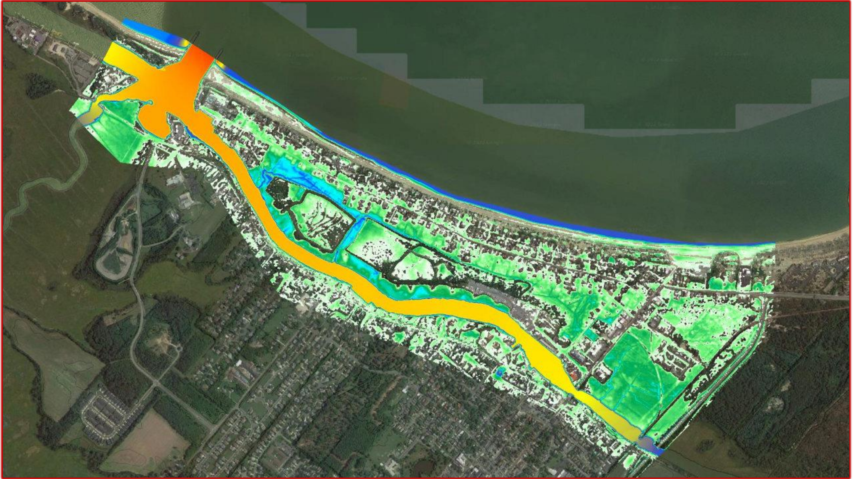
Maximum Tide Elevation 5.0 with Gates Shut at Elevation 2.0 and 5.6-inches Rainfall Added Model
